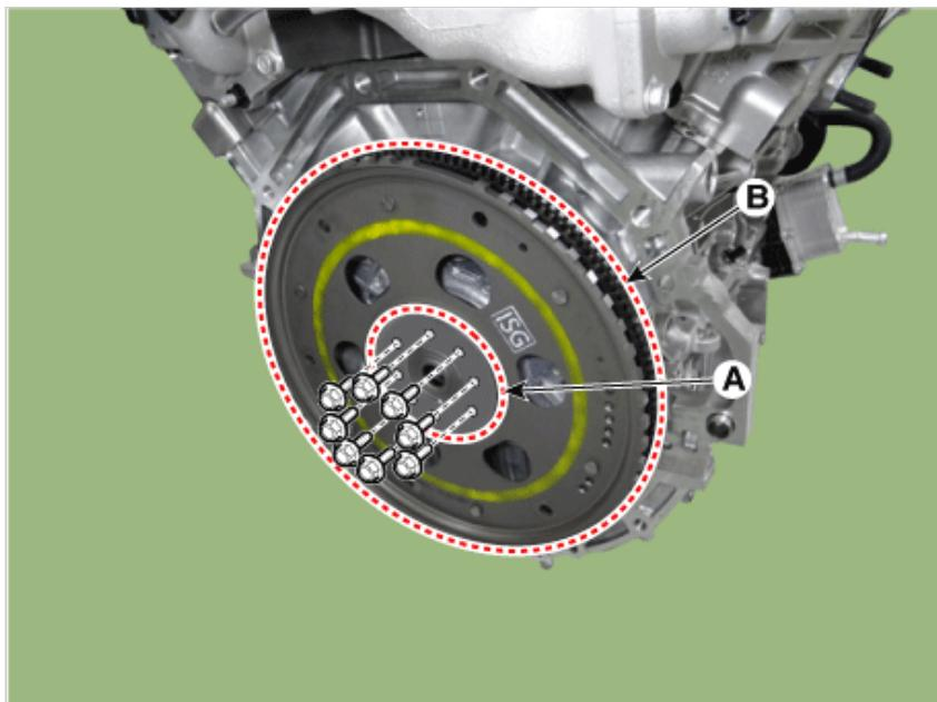
4. Remove the crankshaft adapter (A).
